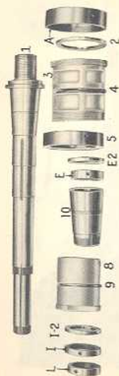
Spindle and Bearings Assembly for 18"-20"-24" Hendey Cone Head Lathes
