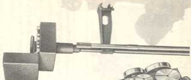
Spring Collet, Closer, and Draw-In Sleeve Assembled Ready for Use in Hendey Motor Driven Cone Head Lathe Spindle
