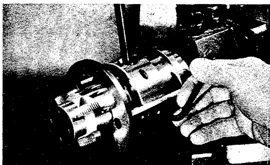
Loosen the trip bar binding screws with the hex key provided.
