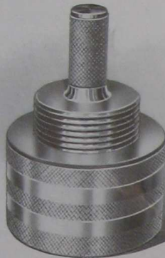
Hardened and lapped master for spindle noses and face plates (Fig. No. 1)
