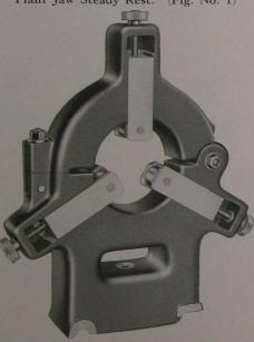
Roller Jaw Steady Rest. (Fig. No. 2)
