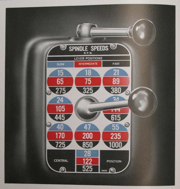
Perhaps the predominant contributing factor to the unprecedented convenience and ease of operation of this new lathe is the newly developed direct reading speed control. This is one of the outstanding features of this new design and is by far the simplest, fastest and most direct reading mechanical control ever furnished on a lathe.
