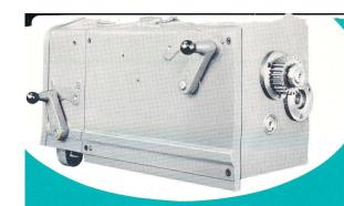
Enclosed quick change gear box. Completely enclosed, lubricated automatically. All gears heat treated and finished. 60 feed and thread changes obtained through exclusive Nebel-designed selector.
