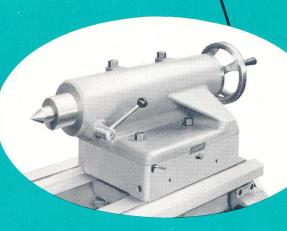
Heavy duty tailstock has 4" diameter spindle, a spindle traverse of 10½", a bearing length of 20" on the bed, and takes a No. 5 ASA standard center. Although the Imperial tailstock weighs 600 lbs., a hook and latch arrangement allows operator to "pick-up" the tailstock and move it with power from the longitudinal feed.
