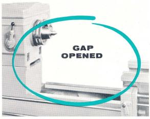
Moving the sliding upper bed to the right opens up a wide, deep gap that will swing outsize work up to 42" in diameter.
