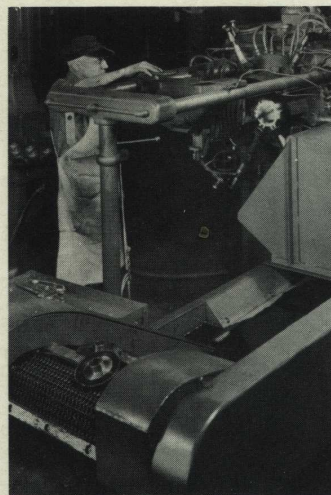
Flame hardening gears
