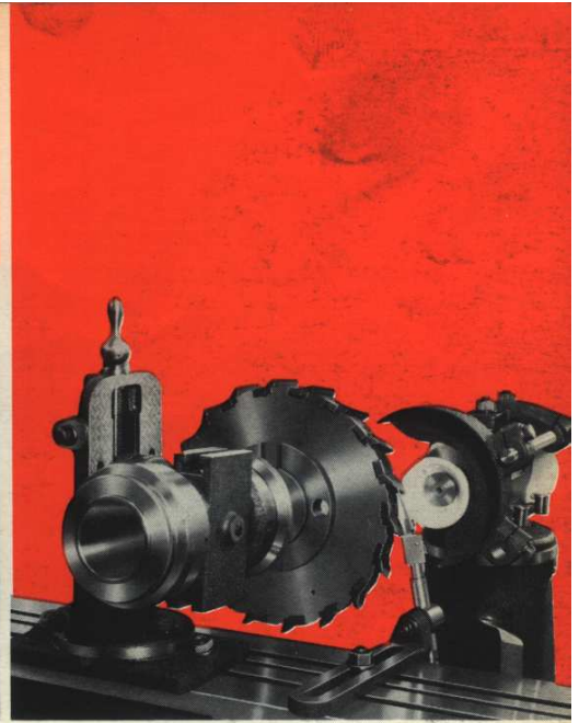
5. FACE MILL: Cutter mounted on tapered shank and held in place in universal work head by an extension arbor same as in a milling machine. Periphery sharpening set-up shown. Easy switch-over for face grinding and beveling.
