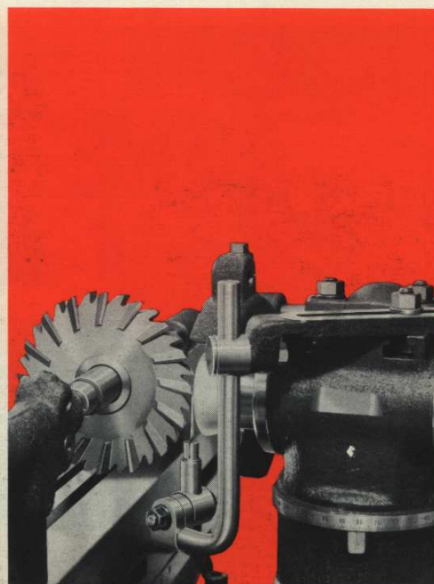
7. STAGGERED TOOTH CUTTER—PERIPHERY: Entire periphery sharpened at one set-up by using universal tooth rest or plain rest with rounded blade, or one with double angles corresponding to those of alternate teeth of the cutter. Rounded tooth rest illustrated.
