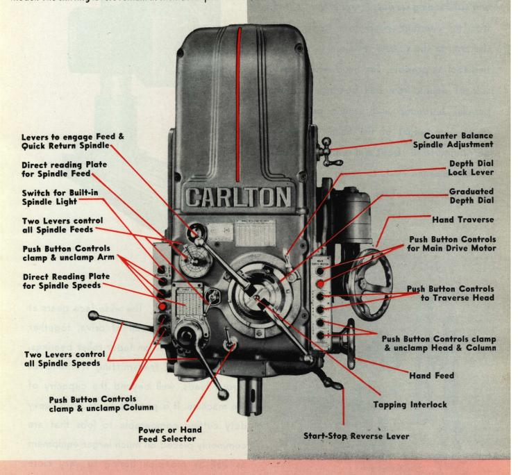
The convenience of the location of these levers has been proven over the past years. Direct reading speed and feed charts simplify shifting problems, although not as fast as the Pre-Select method. The manual shift head can be converted to Pre-Select at a later date, since many of the parts are interchangeable.
