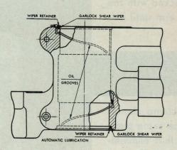
of the arm. These wipers shear the column clean of all foreign material and prevent scoring the arm and column.
