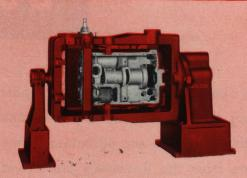
Accurately machined with 4 locating holes for indexing at every 90 degrees. A spring loaded plunger with tapered point is located into a hardened insert. The hole in each insert is ground to the same taper as the plunger for accurate location. The Revolving Stands are available in 20" and 30" sizes. The dimensions are from the bottom face to the centerline of the face plate. End Supports are available for both sizes.
