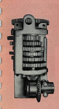
The safety feed clutch is designed to transmit 50% more thrust than the rated capacity of the machine. It will release, with a clicking noise, when taxed beyond its capacity. This clutch prevents overloading, breakage of parts and destruction of valuable tools.
