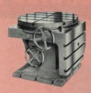
Table tilts 90° — Table top rotates through 360° — Machine graduated in degrees — anti-friction bearing mounting. Table top is available in 32" and 48" diameters. Tee slots are on 6" centers — Mounting slots to base are on 9" centers.
