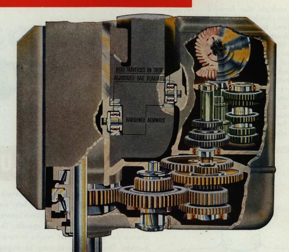
As illustrated above, the Carlton Head is constructed for rigidity and ruggedness. All of the gears that drive the spindle are drop forgings and the spindle is a hammered forging, all made from chrome-moly steel, carburized
