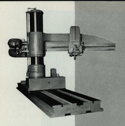
Standard equipment for this unit is non-metallic ways and power traverse. Automatic lubrication to the ways is standard equipment when power clamping is furnished. It is obvious that more stability and precision are available in the sliding base on bedplate than the track type base. Manufacturers of heavy duty machine tools, electrical machinery, large die shops and ordnance have recognized the value of this machine.
