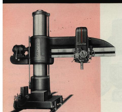
the track itself. The traversing of the machine and the clamping of the machine to the rails are controlled conveniently by two push-buttons mounted on the head.
