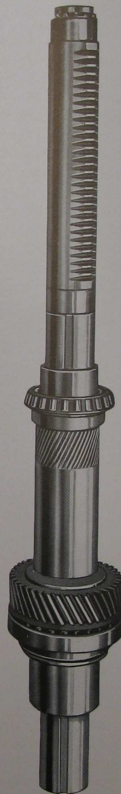
Fig. No. 1 Spindle unit showing integral feed rack, helical gear drive and adjustable Timken roller bearing mounting.
