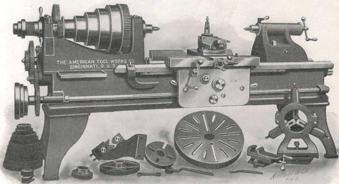
22" Standard Engine Lathe.
